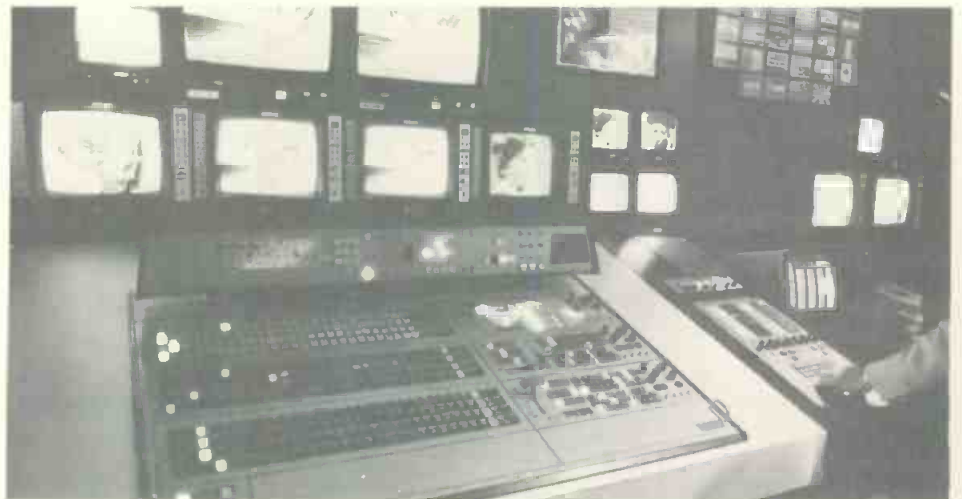
Vital's Saturn Series switcher has four M/Es.
