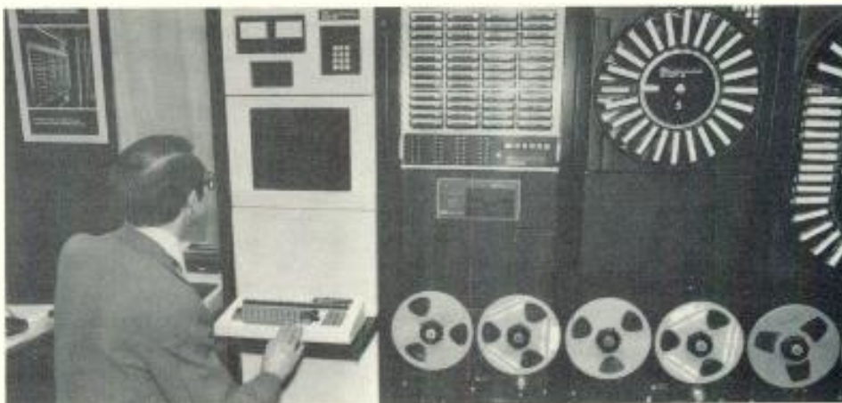
IGM cart equipment under microprocessor control.
